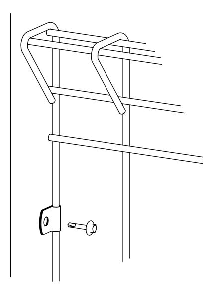
7.5mm steel wire, both horizontal and vertical Hot dip galvanised. Optional powder-coat. Zinc content 300 grams/m2
